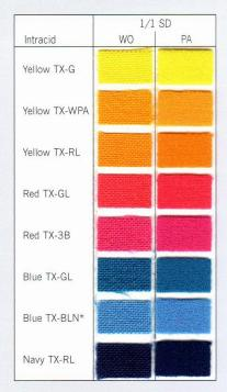
The above dyeings were dyed using 80 parts wool and 20 parts polyamide 6.6, dyed in the same dyebath using the standard dyeing procedure with the addition of Dyapol NDR.
