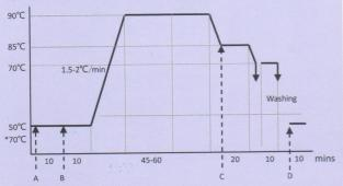
\*For black dyes, the dyeing initial temperature at 70 °C is more advantage to save time.
