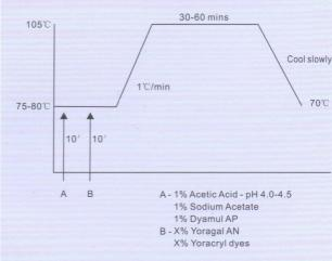
If high temperature equipment is not available, dyeings can be performed satisfactorily at 95-98  $^\circ\! C$
